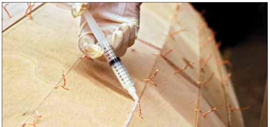
*To accommodate what Harris sees as the progressively diminishing level of experience of would-be amateur boatbuilders, the precisely cut components are optimized for simple construction, including pre-drilled wire holes for the stitch-and-glue method seen here.*
